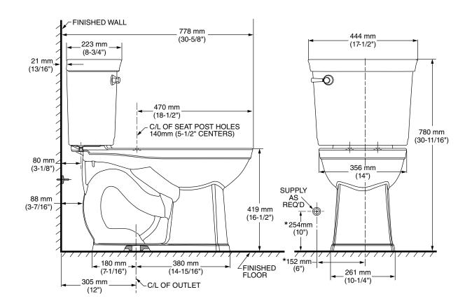
THIS TOILET IS DESIGNED TO ROUGH-IN AT A MINIMUM DIMENSION OF 305mm (12") FROM FINISHED WALL TO C/L OF OUTLET.
