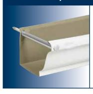
Insert ferrule into gutter and hammer spike through gutter, ferrule and fascia board.
