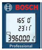
The updated display for the BLAZE™ One allows users to store two measurements on screen for easy calculation of square footage with the simple click of a button.
