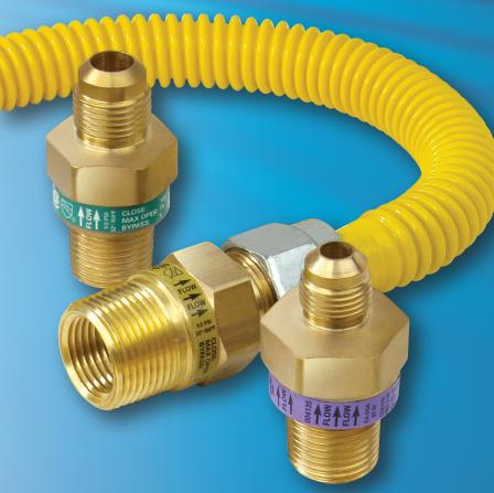
In the event of a gas line rupture or disconnect, unrestricted gas flow forces the diaphragm (1) to firmly position itself against the seat (2). This immediate action restricts gas flow to help avert a hazardous build-up of gas.
