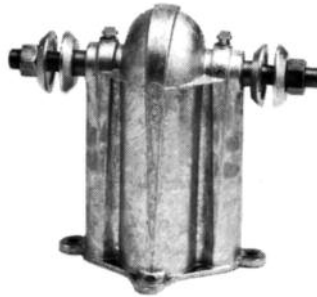
No. 330 SINTERED BRONZE BEARING Shaft length 12" Shaft Diam. 5/8" Pulley Diam. 2" Threaded Ends 1/2" R. & L. V-Belt Size "A" Sec. Shipping Wt. 3 1/4 lbs.
