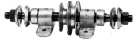
No. 550 SINTERED BRONZE BEARING Shaft Length 9" Shaft Diam. 5/8" Pulley Diam. 2" X 2 1/2" Threaded Ends 1/2" R. & L. V-Belt Size "A" Sec. Shipping Wt. 2 1/4 lbs.
