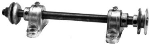
No. 440 SINTERED BRONZE BEARING Shaft Length 12" Shaft Diam. 5/8" Pulley Diam. 2" Threaded End 1/2" L.H. V-Belt Size "A" Sec. Shipping Wt. 3 lbs.
