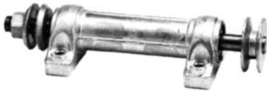
PRECISION BALL BEARINGS No. Shaft Length Diam. Threaded End Wt. 1560 10" 5/8" 5/8" L.H. 3 lbs. Pulley 2" "A" Sec.
