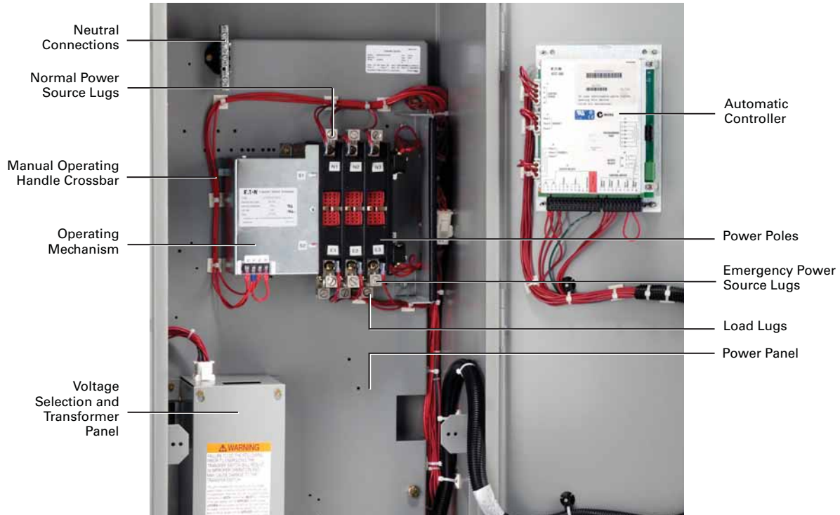
Typical Contactor-Based ATS 100–400 A
