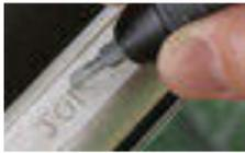
**ENGRAVING CUTTERS** Quality cutters for detail engraving, carving, routing in wood, fiberglass, plastic and soft metals.
