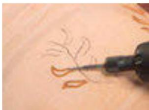
**HIGH SPEED CUTTERS** High speed cutters can be used for shaping, hollowing, grooving, slotting, making tapered holes in soft metals, plastics and woods. # 199 cutter can be used to make small slits.
