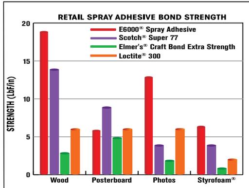
180° Peel Strength Test - ASTM D - 903
