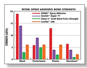
180° Peel Strength Test - ASTM D - 903
