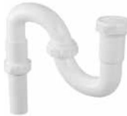
Used in kitchen sink and washbasin applications where plumbing connection is made at floor. Adaptable 1 1/2" x 1 1/4" washer included in P/N 177151. Can be utilized to connect 1 1/2" tubes, 1 1/4" tubes, as well as adapt from 1 1/2" to 1 1/4" tubes.
