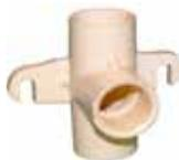
Used on lavatory and sink "rough-ins" instead of conventional tee, providing a more rigid "rough-in" and eliminates the need for tubing hangers. Also provides for rigid mounting of washer valves for automatic washer hose hook-ups at laundry tray.
