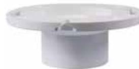
Solvent welds over 3" Sch. 30 pipe. Unique "Pop-Top" feature prevents debris from entering plumbing system prior to setting the toilet. Used for mounting toilet base to drain.
