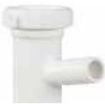
Used for hooking up automatic dishwasher drains to exposed sink drains in installations not employing garbage disposal. Branch accepts 7/8" I.D. hose or rubber dishwasher drain connectors
