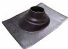
These weatherproof thermoPlastic flashings, featuring a replacement boot, provide seal around plumbing vent pipes. Manufactured totally from corrosion proof materials. They eliminate shingle staining problems. Can be used on all types of plumbing pipes and electrical conduit. Base dimensions (14661) 8½" X 11¾", (14562-64) 12" X 16".
