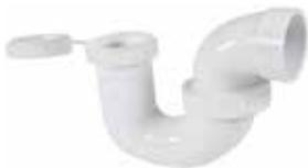
Used to prevent the passage of sewer gas from the plumbing system into house through the plumbing fixture drain. Used when local code doesn't permit the use of slip coupled traps.
