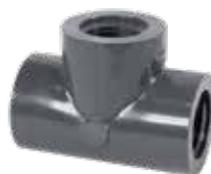
Adapts to male threaded main line to provide a threaded branch line of the same size. PTFE thread tape is recommended for threaded joints.
