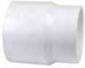
This fitting adapts Genova Sch. 40 pipe to 4" cast iron spigot and can be joined to cast iron with oakum and poured lead or poured lead substitute.
