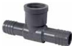
Used to provide a branch supply line from a main line. Branch line adapts to standard male pipe threads. PTFE thread tape is recommended for threaded joints.
