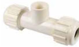
Provides a threaded branch line from a main line. Adapts PVC pipe or other iron pipe sized pipe to male pipe threads in cold water applications. PTFE thread tape is recommended for threaded joints.
