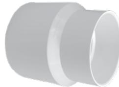
This fitting adapts 3" Sch. 30 pipe to 3" cast iron spigot. Can be joined to cast iron with oakum and poured lead or lead substitute.
