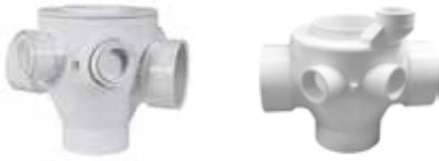
Provides for the hookup of all drains from two complete bathrooms located back to back. Each unit furnished with two flush branch plugs to enable utilizing the fitting in a left or right hand drain situation. Branch inlets are 2" socket configurations to accept 2" pipe. Bushing (Part #70221) are provided to accommodate 1½" pipe.
