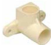
This elbow is used to change direction in piping and features lugs for fastening. Often used in conjunction with Washer Hose Valve (#530671) for hooking up to automatic clothes washers as well as fabricating water supply piping stub outs for toilet installation. Sometimes called a "Drop Ear" elbow.
