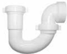
Adaptable 1 1/2" x 1 1/4" washer included. Can be utilized to connect 1 1/2" tubes, 1 1/4" tubes, as well as adapt from 1 1/2" to 1 1/4" tubes. Furnished with special PVC elbow to allow solvent welding directly to 1 1/2" Sch. 40 pipe.
