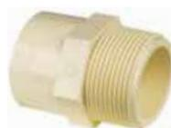
Used to adapt female pipe threads to CPVC tubing in COLD WATER APPLICATIONS ONLY! Where hot water or changing water temperatures are likely to be encountered, utilize the recommended TRANSITION UNIONS. PTFE thread tape is the accepted method of sealing pipe threads on CPVC fittings. Do not use other materials or compounds unless specifically approved by the manufacturer.
