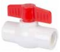
These ball valves are made out of PVC for corrosion resistance. Used anywhere a full flow valve is required, such as swimming pools, irrigation systems or agricultural applications. Adapts to standard male pipe threads. PTFE thread tape is recommended for threaded joints. Working Pressure: 150 PSI @ 73°
