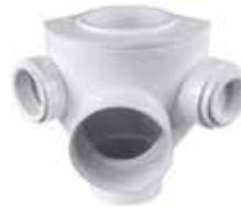
This special stack fitting provides for the hookup and venting of a complete bathroom. Each unit includes a flush branch plug to enable utilizing the fitting in a right or left hand drain situation. Branch inlets are 2" socket configurations to accept 2" pipe. Bushings (Part #70221) are provided to accommodate 1½" pipe.
