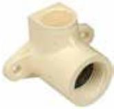
This elbow adapts from ½" CPVC to ½" male metal pipe threads and features lugs for fastening. A special elastomeric gasket ensures a leakproof seal. Used on tub and shower faucets to adapt from the ½" CPVC riser to the chrome shower arm. Sometimes called a "Drop Ear" elbow.
