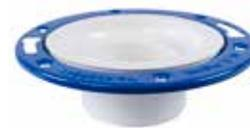
Solvent welds directly into 3" Sch. 30 fitting hub. This flange has an adjustable metal ring which allows for easier toilet alignment.
