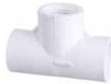
Solvent welds into main line to provide a threaded branch line of the same size. PTFE thread tape is recommended for threaded joints.
