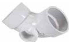
Used to connect a branch line or vent at a change of direction in a larger vertical or horizontal pipe. The inlet is constructed to accept a 2" fitting over its outside diameter or 1½" pipe into its inside diameter.
