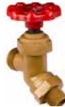
For use with female threaded fitting in cold or hot water up to 150 PSI @ 180°F. (3/4" hose thread) PTFE thread tape is recommended for threaded joints.
