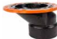
This flange has an adjustable metal ring which allows for easier toilet alignment. Solvent welds over 3" Sch. 40 pipe.
