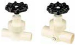
This unique valve employs the globe valve principle and is manufactured of high temperature thermoplastics. It is designed to solvent weld to CPVC tubing. This valve employs "Street/Socket" feature which allows it to be used with 1/2", 3/4", and 1" CPVC tubing. (2 - 3/4" couplings are required to attach the valve to 3/4" CPVC tubing. 2 - 1" couplings are required to attach the valve to 1" CPVC tubing).
