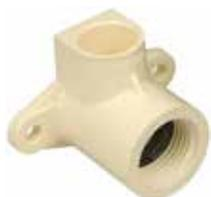
This elbow adapts from 1/2" CPVC to 1/2" male metal pipe threads and features lugs for fastening. A special elastomeric gasket ensures a leakproof seal. Used on tub and shower faucets to adapt from the 1/2" CPVC riser to the chrome shower arm. Sometimes called a "Drop Ear" elbow.
