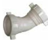
Adaptable 1½" x 1¼" washer included. Can be utilized to connect 1½" tubes, 1¼" tubes, as well as adapt from 1½" to 1¼" tubes. Coupler allows for changes in direction and realignment of exposed tubular piping.
