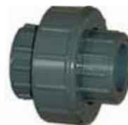
This union solvent welds directly to PVC pipe and provides a method for future disassembly of piping without cutting. Working Pressure: 150 PSI @ 73°
