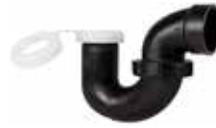
Used to prevent the passage of sewer gas from the plumbing system into house through the plumbing fixture drain. Used when local code doesn't permit the use of slip coupled traps.
