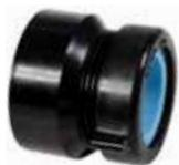
Utilized to adapt ABS pipe to tubular traps at wall or floor. This fitting solvent welds over 1½" DWV pipe. Sometimes called a Marvel.
