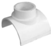
Solvent welds directly to side of sewer pipe to provide a simple way of connecting a branch into a drain pipe. The inlet is constructed to accept a 2" fitting over its outside diameter or a 1½" pipe into its inside diameter.
