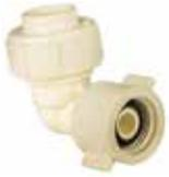
Allows a direct 90° connection between 5/8" O.D. PEX, copper, or CPVC tubing and male running threads on faucet. Has a cone washer inside female end to achieve seal.
