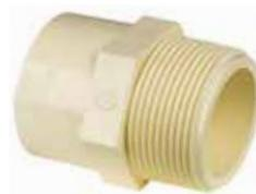
Used to adapt to metal FIP threaded fittings in COLD WATER APPLICATIONS ONLY! Where hot water or changing water temperatures are likely to be encountered, utilize the recommended TRANSITION UNIONS.
