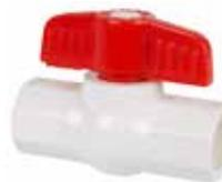
These ball valves are made out of PVC for corrosion resistance. Used anywhere a full flow valve is required, such as swimming pools, irrigation systems or agricultural applications. Working Pressure: 150 PSI @ 73°
