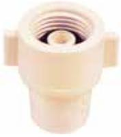
Allows a direct connection between supply tube and male running threads on faucet. Has a cone washer inside female end to achieve seal.
