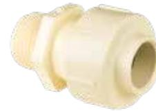
Designed to adapt from metal female pipe thread to PEX, copper, or CPVC tubing on the COLD WATER SIDE ONLY of a hot and cold water supply system. Where hot or changing temperatures are likely to be encountered, utilize a short metal nipple in conjunction with a Genova Universal Fitting Special Female Adapter. PTFE tape is the accepted method of sealing pipe threads or CPVC fittings. Do not use other materials or compounds unless specifically approved by the manufacturer.
