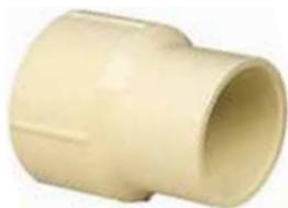
Used to adapt metal FIP threaded fittings to CPVC. A special elastomeric gasket ensures a leakproof seal. Hand-tighten only! This fitting seals by means of a gasket. The use of joint compound or Teflon tape is neither necessary or recommended.
