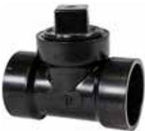
Used at the base of a vertical drain pipe to provide a cleanout opening flush with the finished wall. PTFE thread tape is recommended for threaded joints.
