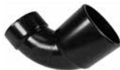
Used to change direction in piping as well as size. Usually utilized to convert from 3" horizontal pipe to 4" fitting hub directly under the toilet.
