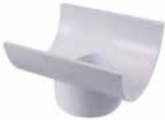
Solvent welds directly onto the side of a 3" pipe to provide a simple way of connecting a branch into a drain pipe. The inlet is constructed to accept a 2" fitting over its outside diameter or a 1½" pipe into its inside diameter.
