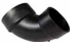
Used to change direction in piping as well as size. Usually utilized to convert from 3" horizontal pipe to 4" vertical pipe directly under the toilet.
