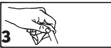
Fig. 1 Using Genova Plastic Tubing Cutters (PN 53499), cut tubing squarely to length.
