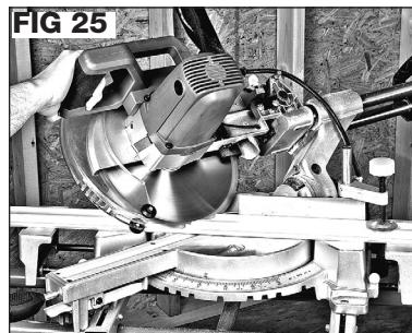
1. Set the bevel angle and miter angle as described earlier and lock the respective adjustment handles securely.
