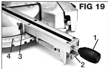
**NOTE:** This miter saw comes with 9 positive stops: 0° for 90° cutting, left-15°, 22.5°, 30°, 45°, right-15°, 22.5°, 30°, 45° for quick setting of common miter cutting angles.
