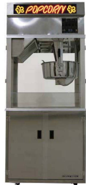
#2911 52 oz. Kettle, 36" Cabinet (shown) 36"W x 28"H x 84"D (91 x 71 x 213cm), 8030 watts, 50 am plug, 120/208 - 120/240 volts.
