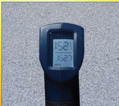
Uncoated white granulated roof = 152°F
