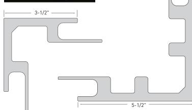
**Kieer Konceal** has a built-in 3/4" reveal that covers rough cuts at corners and other areas where precision cuts are time consuming and difficult. Meaning you save time without sacrificing that striking, finished look. Suitable for use with vinyl, fiber cement or wood siding, Kleer Konceal is available in smooth or natural woodgrain textures that ensure appealing aesthetics and lasting value.
