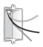
3-wire Separate wires for fan and light
