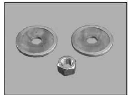
(O) Clean the Inner and Outer Flanges and the Blade Retaining Nut.
