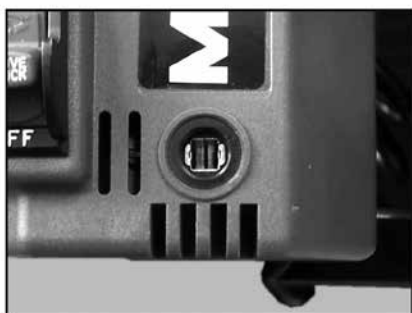
(D) Clean the Motor Brush Housing using a Q-tip.
