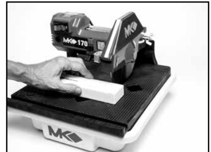
(F) Push the Dressing Stick into the Blade in a smooth even mo- tion to perform a cut, repeat 7 or 8 times to dress the Blade.
