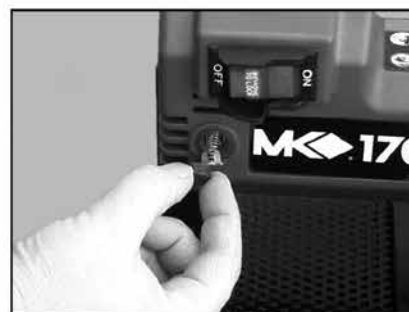
(C) Remove Motor Brush Housing Cover.
