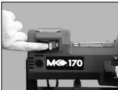
(A) Check the ON/OFF Switch is in the ON position.
