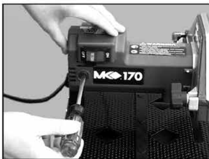
(B) Locate and Remove One Motor Brush Cap using a Flat Head Screwdriver.
