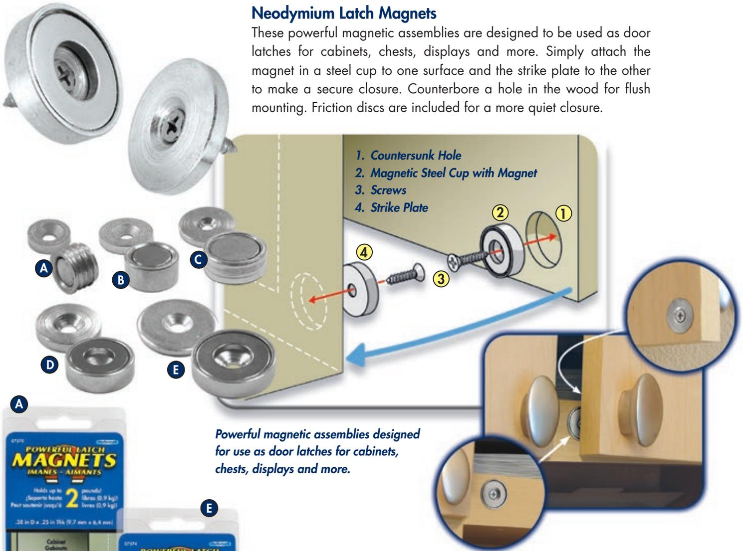
Powerful magnetic assemblies designed for use as door latches for cabinets, chests, displays and more.
