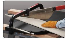
Scribe desired angle on fiber cement siding plank and feed it into the quillotine blade as you cut.
