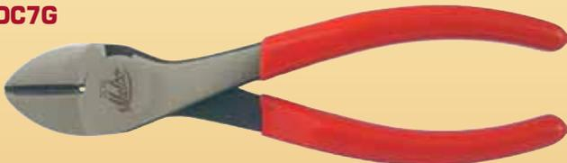
Powerful leverage short nose is designed to cut flush from side without obstructing handle grip. Absence of flat gripping surface on jaws allows tool to cut out to very tip. (Diagonal cutters are the only tools capable of reaching into an electrical box to cut wires). Smooth functioning box joint insures accurate alignment of cutting edges. Forged from high quality alloy steel. Hardened and tempered for long life. Polished faces. Red vinyl cushion grips.
