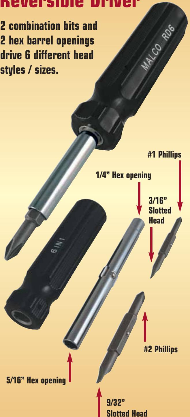
Bit shank firmly locks into handle barrel. Driver bits are individually protected with black oxide. Barrel is chrome plated to protect against rust.
