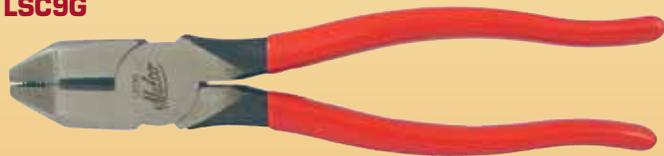
High leverage plier is designed for cutting number 8 and other large wires. Forged from high quality alloy steel. Precision matched cutting edges are induction hardened. Jaw rivet is offset for increased leverage. Built-in insulation crusher. Red vinyl cushion grips.
