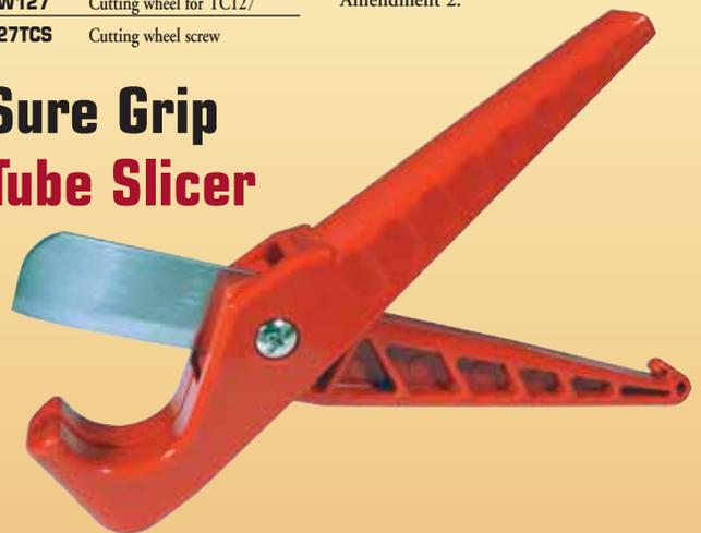
Produces cuts in ABS, PVC, rubber and fabric reinforced hose up to 1" (25.4 mm) I.D. Rigid, durable nylon handle design provides sufficient leverage when cutting so that only moderate hand pressure is required. Stainless steel cutting blade is resharpenable and replaceable.
