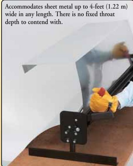
Accommodates sheet metal up to 4-feet (1.22 m) wide in any length. There is no fixed throat depth to contend with.
