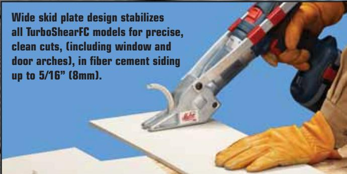
Wide skid plate design stabilizes all TurboShearFC models for precise, clean cuts, (including window and door arches), in fiber cement siding up to 5/16" (8mm).
