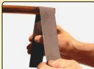
Creates a bite on metal surface for solder or paint. Aluminum oxide cutting grain rates 9.2 on MO scale (diamond=10). Flexible cloth back fits contours of any surface configuration and hard to reach areas. Long lasting urea resin bonding is water resistant.
