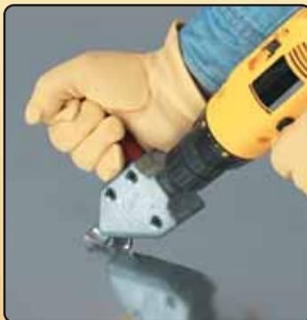
For best results, be sure to keep the **TURBOSHEAR** blades level with cutting plane, this offset design also keeps hands away from work surface.
