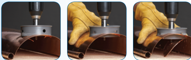
Outlet Saw cutting progression in half round gutter.
