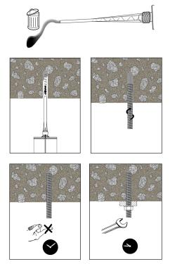
Note for decreased installation temperature: When installing CIA-EA at decreased installation temperature  $(+32^{\circ}F < T < +50^{\circ}F (0^{\circ}C < T < +10^{\circ}C))$ the cartridge must be conditioned to  $+68^{\circ}F (+20^{\circ}C)$ .
