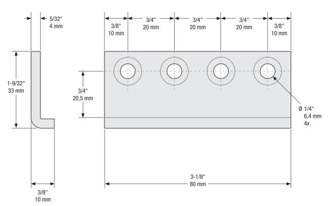
Material: Steel Finish: Oil Rubbed Bronze Fasteners: (4) Hex Socket Screw, M6 x 3/8" Long, Countersunk
