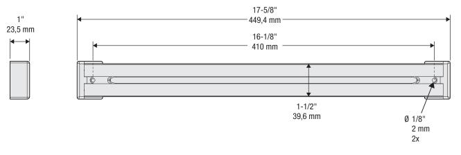
Material: Steel Finish: Gray Powder Coating SWL: 3 lbs Fasteners: (2) #6 x 1-1/2" Long Type A, Phillips, Round head (2) Anchor Pilot hole: 3/32"
