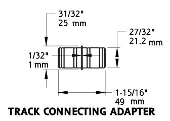
Material: Stainless Steel Fasteners:(2) Phillips Screw, Flat Head M6 X 75 mm
