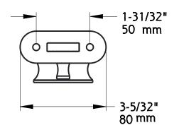
Material: Stainless Steel Fasteners: (2) Hex Screw, M6 x 1-3/16" Long (2) Screw Anchor, M6 x 1" Long
