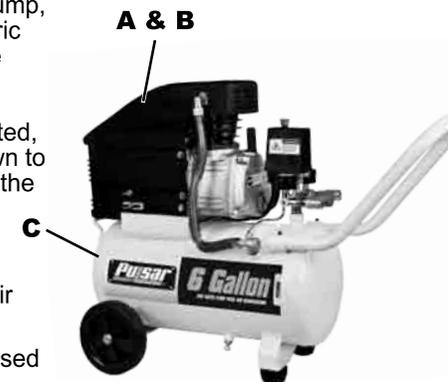
The pump (see B) compresses the air and discharges it into the tank.
