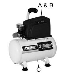
The pressure switch (located internally) shuts down the motor and relieves air pressure in the pump and transfer tube when the air pressure in the tank reaches the kick-out pressure. As compressed air is used and the pressure level in the tank drops to the kick-in pressure, the pressure switch restarts the motor automatically, without warning, and the pump resumes compressing air.
