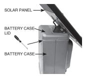
Solar panel is riveted to battery case lid. The battery case lid is attached to the battery case by friction. Using a flat head screwdriver lift battery case lid just above the raised ridge of battery case. Carefully remove the battery case lid with solar panel to expose battery inside battery case. There may be cardboard packing inside the battery case used to keep the battery from shifting during shipment. Replace cardboard after installing new battery.
