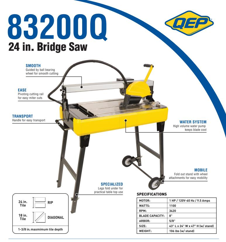
The QEP 24 inch Bridge Saw evenly distributes water flow, extending the life of the diamond blade. The ball-bearing cutting assembly ensures the user a smooth score leading to cleaner accurate cuts, and a fold-out stand with wheel attachments for easy mobility and storage. Power cords are encapsulated in a protective tube and attached to a flexible rod that keeps the cutting table safe and clear. Comes with a one year limited warranty.
