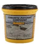
**Curing:** QUIKRETE® Concrete Patching Compound will form a surface skin in 20 – 40 minutes and will become hard in 4 – 6 hours depending on temperature and humidity. Additional curing will continue for about 3 days, longer under low temperature and high humidity conditions.
