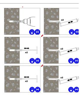
If the hole collects water after the initial cleaning, this water must be removed before injecting the resin.
