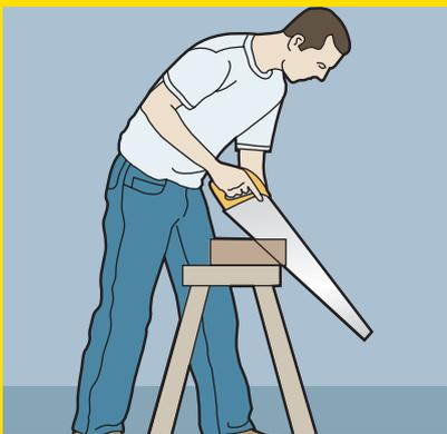
the saw cutting edge angled at approximately 30° to the work surface. Use the thumbnail of the hand not holding the saw, or a scrap piece of wood, position the cutting edge to the waste side of the line. The first stroke should be a light pull to establish the cutting line (kerf).
