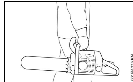
**By hand:** When transporting your chain saw by hand, the engine must be shut off and the chain saw must be in the proper position, i.e., grip the top handle and place the muffler away from the body; the chain guard (scabbard) should be over the saw chain and guide bar, which should point backwards, away from the direction in which you are walking.
