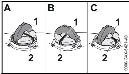
If the cap does not drop fully into the fuel tank opening when the positioning marks (1, 2) line up, or if it does not tighten properly when turned, the base of the cap may be prematurely rotated in relation to the top. Such misalignment can result from handling, cleaning or an improper attempt at tightening.
