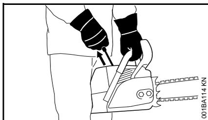
The **second** recommended **method** for starting your chain saw allows you to start the saw without placing it on the ground. Make sure the chain brake is engaged, grip the front handle of the chain saw firmly with your left hand. Keep your arm on the front handle in a locked (straight) position. Hold the rear
