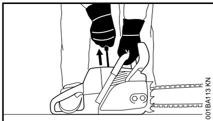
With the **first** recommended **method**, the chain saw is started on the ground. Make sure the chain brake is engaged (see "Chain Brake" chapter in your instruction manual) and place the chain saw on firm ground or other solid surface in an open area. Maintain good balance and secure footing.
