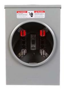
Siemens Low Voltage Talon Meter Sockets Residential - Talon Meter Sockets UAT1 Steel are Residential Enclosures Single-Family Metering. Type: UAT1 Special Features: NO BYPASS Application: RESIDENTIAL Standard: UL Voltage Rating: 300V Amperage Rating: 135A Phase: SINGLE PHASE Size: 4.900X8.700X13.300 Cable Entry: OH/UG Terminal: 4 TERMINALS Mounting: SURFACE MOUNTING Operating Temperature: AVERAGE AMBIENT Enclosure: STEEL
