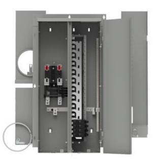
SIEMENS LOW VOLTAGE METER LOAD CENTER COMBINATION. FACTORY INSTALLED MAIN BREAKER 20 (1 INCH) SPACES INTERIOR ALLOWING MAX 40 CIRCUITS. 4-JAW METER / 1-PHASE SYSTEM RATED 200A. SPECIAL FEATURES: OH/UG FEED, RING TYPE COVER, FLUSH MOUNTING, EUSERC APPROVED
