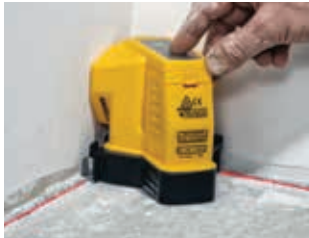
Positions inside corners to check for square
