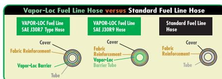
HBD/Thermoid's VAPOR-LOC Barrier System is currently available on fuel line hoses and bulk fuel /bio-fuel transfer hose products. The close-up photo of this Thermoid Transporter Bio-Fuel
