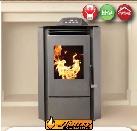
AP5710 Pellet Stove 48,000 BTU's, 2,200 Sq. Ft. 20 lb. Capacity, 100 CFM Blower 1.03g/hr, Digital Controls, 160 lbs.
