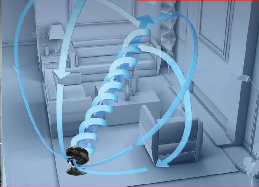
**A Vornado circulator differs from a regular fan by using Vortex Action to distribute air throughout the entire room.** Vortex Action refers to the column of air that circulators create. The airflow column will spin and twirl to the opposite corner hitting the wall where it will split off and recirculate to the centre of the room. Whole room circulation means that you don't have to be directly in the air stream of the circulator to feel its effects.
