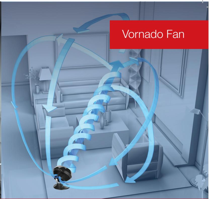
**A Vornado circulator differs from a regular fan by using Vortex Action to distribute air throughout the entire room.** Vortex Action refers to the column of air that circulators create. The airflow column will spin and twirl to the opposite corner hitting the wall where it will split off and recirculate to the centre of the room. Whole room circulation means that you don't have to be directly in the air stream of the circulator to feel its effects.
