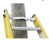
Slip-resistant rubber grip attached to steel v-rung for wood, metal or concrete poles. Pre-pierced holes in fiberglass top rails are provided to accept this accessory. V-rung assembly comes with mounting hardware and instructions.
