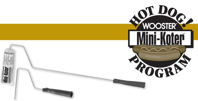
STANDARD MINI-KOTER FRAMES Blue plastic grips, threaded for extension pole use. Sturdy wire shanks have a chamfered end to enable them to be more universally used with competitive covers. R127–R129 have high-capacity rollers for all flat paints and stains. Roller not included with the R029 frame—customize with any of the Mini-Koter packs.
